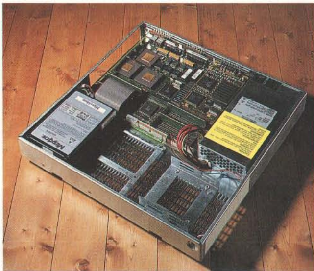
Photo 2: The Trimm case has enough room to mount two internal 3½-inch hard drives and a 3½-inch floppy drive. The Integrix color SBus display adapter is pictured on the right side.
